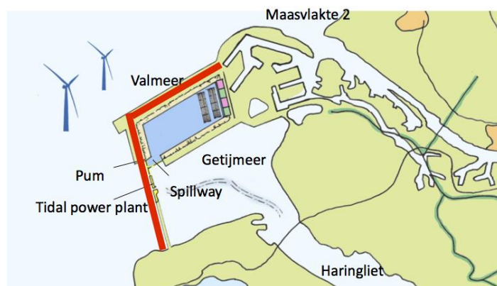
Figure 10: The new flood protection by the DELTA 21 project
