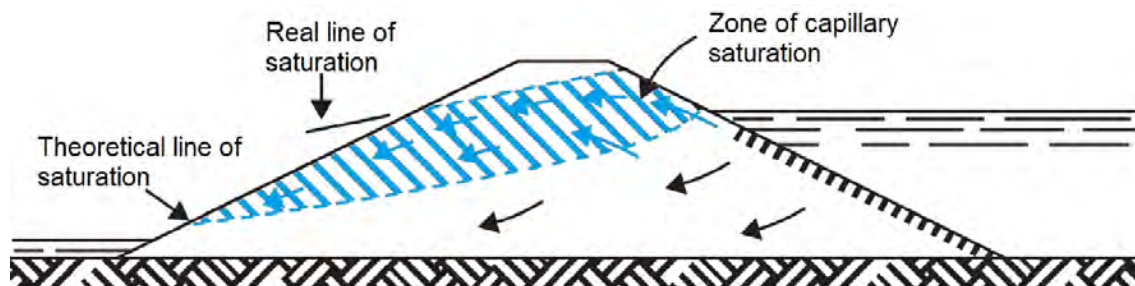
Figure 2.1: A dike illustrating the flow of water above the theoretical phreatic line through the capillary zone (Terzaghi, 1943)
