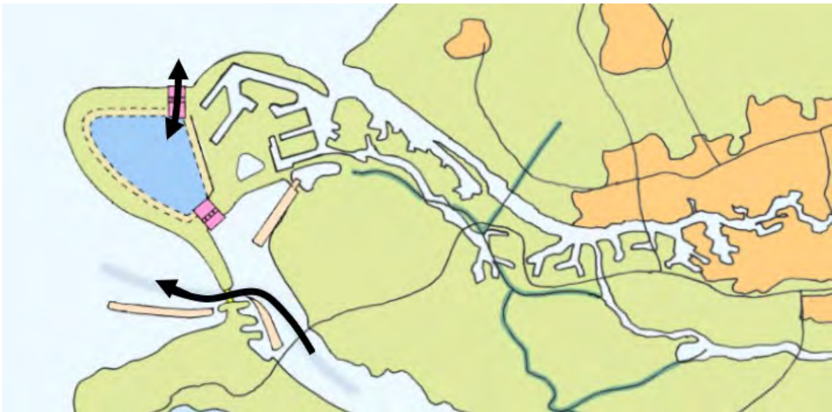
Figure 2.5: Map of the Delta21 waterdefence system (black arrows represent direction of water flow at normal conditions)(Lavooij et al., 2018)
