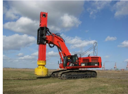
Figuur 24.: Cofra Dynamic Compaction
