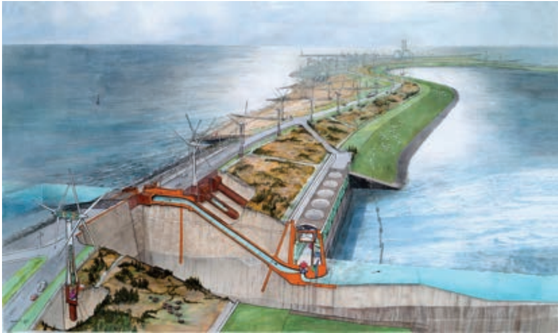
Figure A.6: Dike section of the Valmeer with the pumping system (Illustration by the Das brothers). Source: https://www.deingenieur.nl/artikel/lievens-de-man-van-het-opslagbekken
