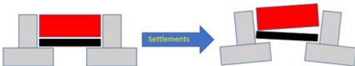
Figure H.1: Settlements affection to closing operation for the Eastern Scheldt barrier.
