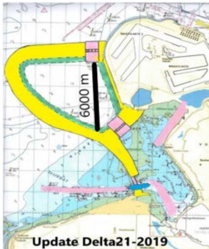
Figure F.1: Largest distance for wind wave generation hitting the power plant
