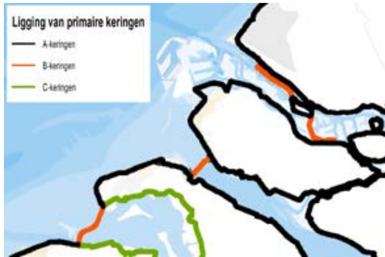
Figure 3.1: Location of a, b and c barriers in the system of primary flood defenses
