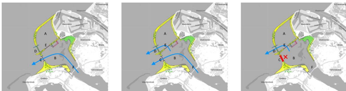
FIGURE 4: NORMAL CONDITIONS (LEFT), HIGH DISCHARGE (MIDDLE), HIGH WATER LEVEL AT NORTH SEA (RIGHT) (ADJUSTED FROM: LAVOOIJ AND BERKE (2020))
