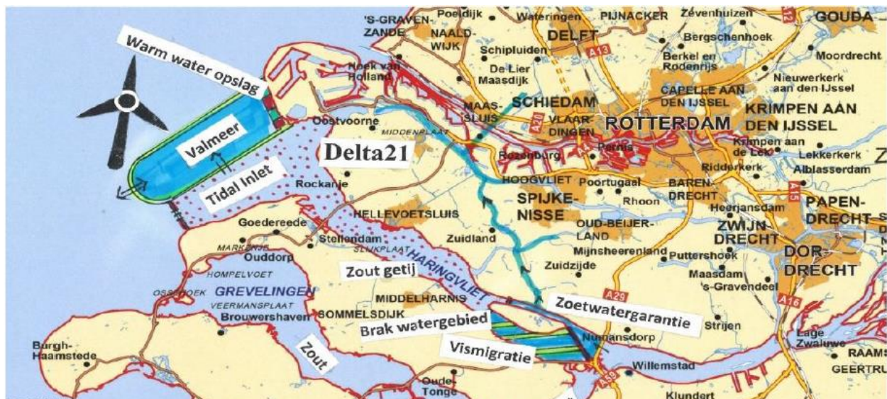
Figure 1. Span of the Delta21 works (Delta21, 2017)
