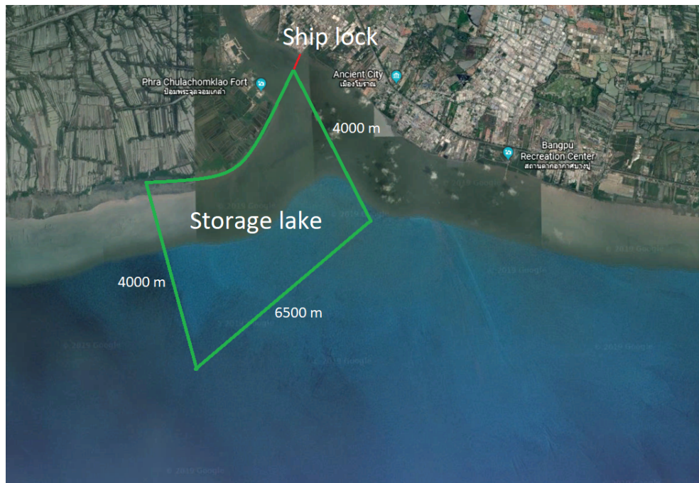
Figure C.2: First design DELTA21 in Bangkok with some dimensions
