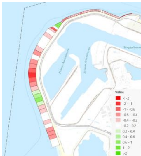
Figure 6.13: Bathymetry changes in meters between 2013Q2 and 2014Q2 for the profile between +3m NAP and -4m NAP. Red indicates a bathymetric decrease of the bottom profile, green indicates an increase. Visualisation in ArcGIS. Data-source: PUMA
