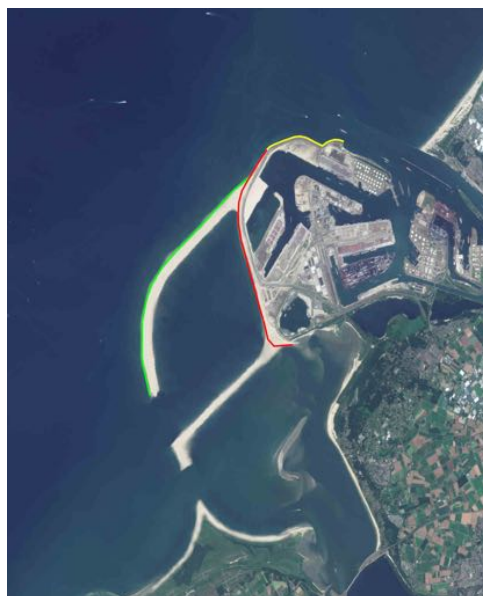
Figure 2.1: The research area of this thesis. The current soft sea defence of Maasvlakte 2 in red, the current hard sea defence in yellow and the to be researched soft sea defence of Delta21 in green.
