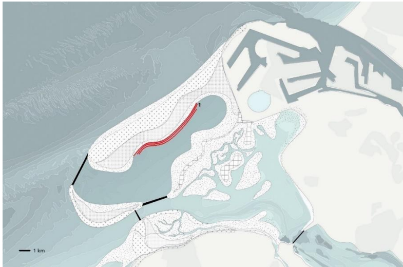
Figure 9. The layout of the lake by Esmee adapted to our advice. The number 1 represents the location of the SeaStairs where for example, seagrass meadows or the permanently flooded sandbanks can be restored.
