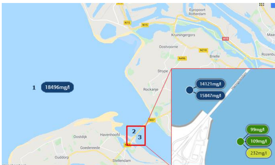
Figure 9. Salinity level of the water in the Haringvliet delta at different locations and depths (at 29-01-2020). The levels at location 2 represent the upper and lower water layer. The values at location 3 represent the salinity level at respectively 2, 6, and 11 m water depth. Source: Rijkswaterstaat Waterinfo (2020a).
